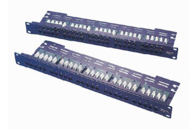
KUWES ISDN patch panel utilizes printed circuit design to provide high performance and flexible application. Offering 25 or 50 port panel for ISDN or Cat.3 wiring system. The design of the PCB provides connection for data or voice application on pin 3,4,5,6 of the RJ45 Jacks. 4 different terminal options are available.
